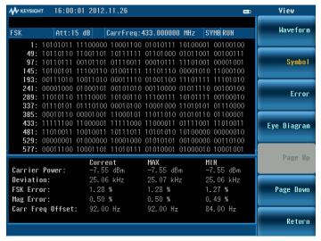
Figure 7. FSK demodulation with symbol view
