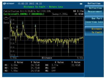
Figure 10. Measuring distance-to-fault with N9322C
