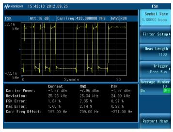
Figure 5. FSK demodulation with waveform view
