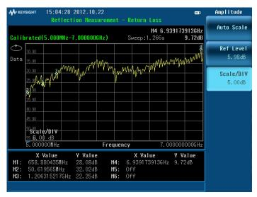
Figure 11. Measuring return loss with N9322C
